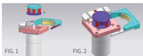
Install the roller parts (purple part) vertically downwards as shown in Figure 1 Flat installation to make sure purple part share the same plane with the pink part.
